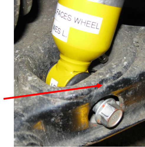
Rear shock installed, Schrader valve (mostly hidden) toward axle
