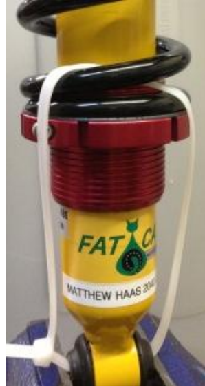
FCM Elite coil-over, typical spring perch location, as shipped.
