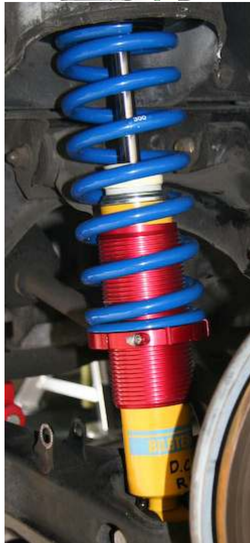
FCM custom coil-overs, front and rear, typical spring perch locations, as shipped.
