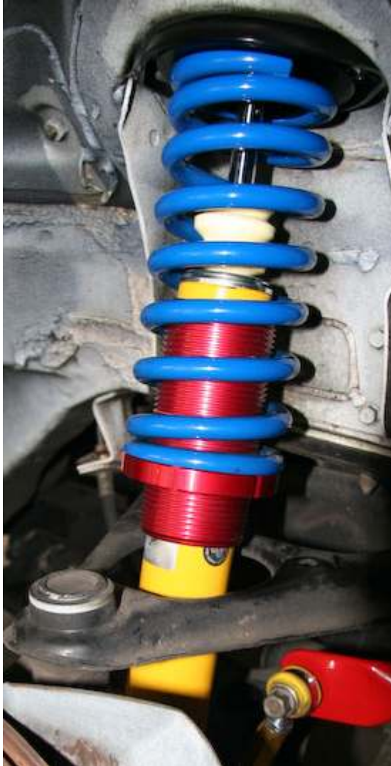
FCM custom coil-overs, front and rear, typical spring perch locations, as shipped.
