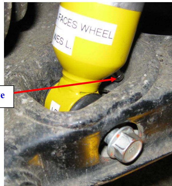
Rear shock installed, Schrader valve (mostly hidden) toward axle
