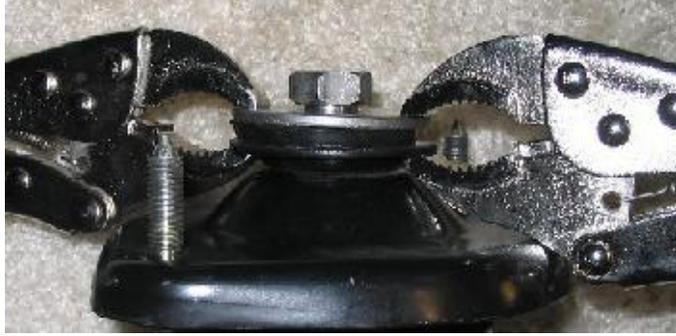
Without an impact wrench, there will be more resistance as the nut turns so you will have to use stronger means to keep the shaft from spinning. A strap wrench works well, as does a mouse pad or other thick, high-friction material held inside pliers, etc. **Whatever your approach, be sure the shaft does not spin as this may damage internal seals.**
