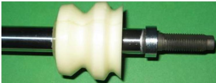
Upper spring isolators, cupped washer and shock mount assembly
