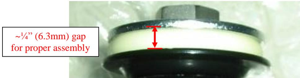
12. Ensure the gap is about 1/4" and the bushings are still centered in the shock mount.
