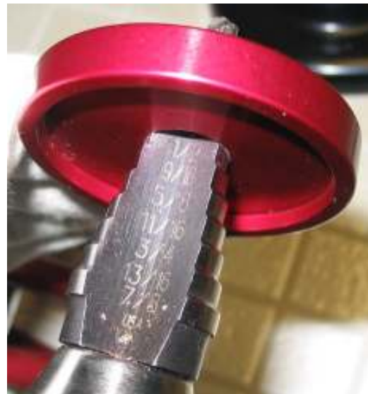
Supplied cupped washer, shown drilled for Koni
