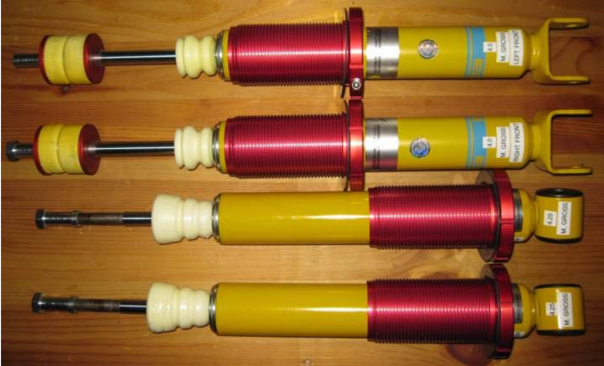
Figure 1a. Unassembled NC (2006+) MX5 Miata FCM Variant 2 coilovers. MCU bushing (in yellow) shown on upper portion of front shocks – not provided in all cases
