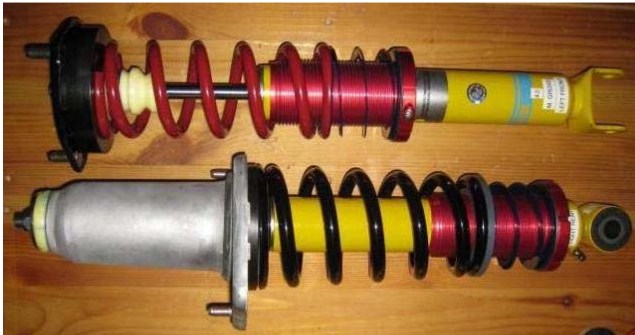
Figure 1a. Unassembled NC (2006+) MX5 Miata FCM Variant 2 coilovers. MCU bushing (in yellow) shown on upper portion of front shocks – not provided in all cases
