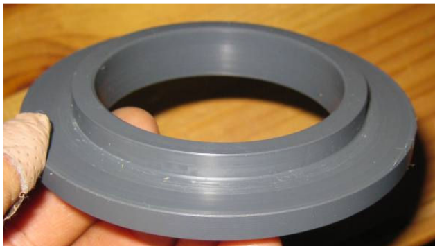
Figure 15. Rear spring adapter, top shown For 70mm ID main spring
