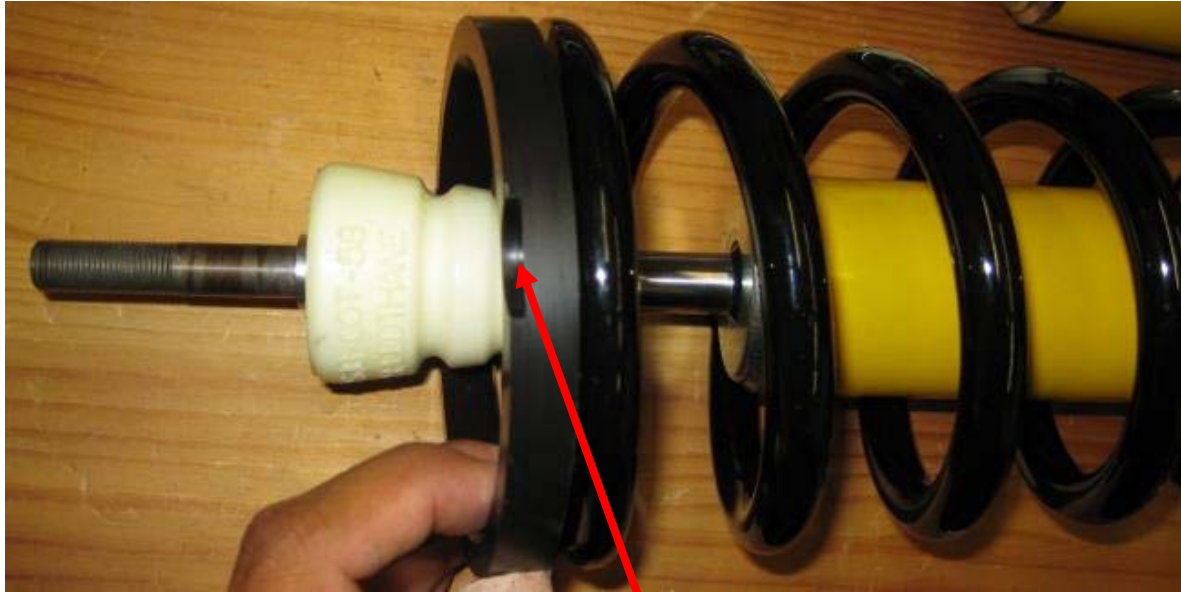
Figure 19. Rear upper spring adapter (note notch) placed on 70-90mm main spring
