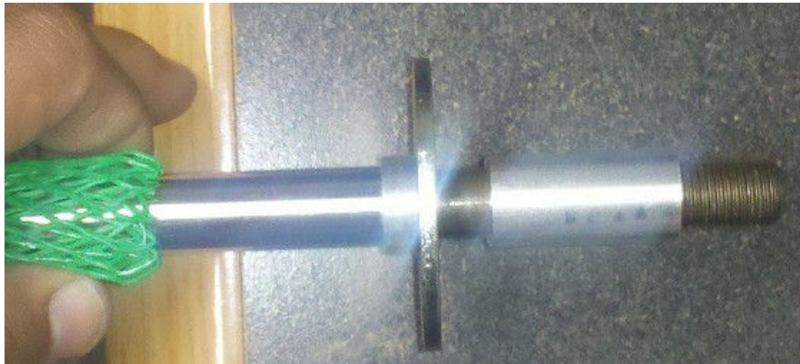
Figure 7. The FCM aluminum bushing sleeve replaced the OE zinc-plated bushing sleeve
