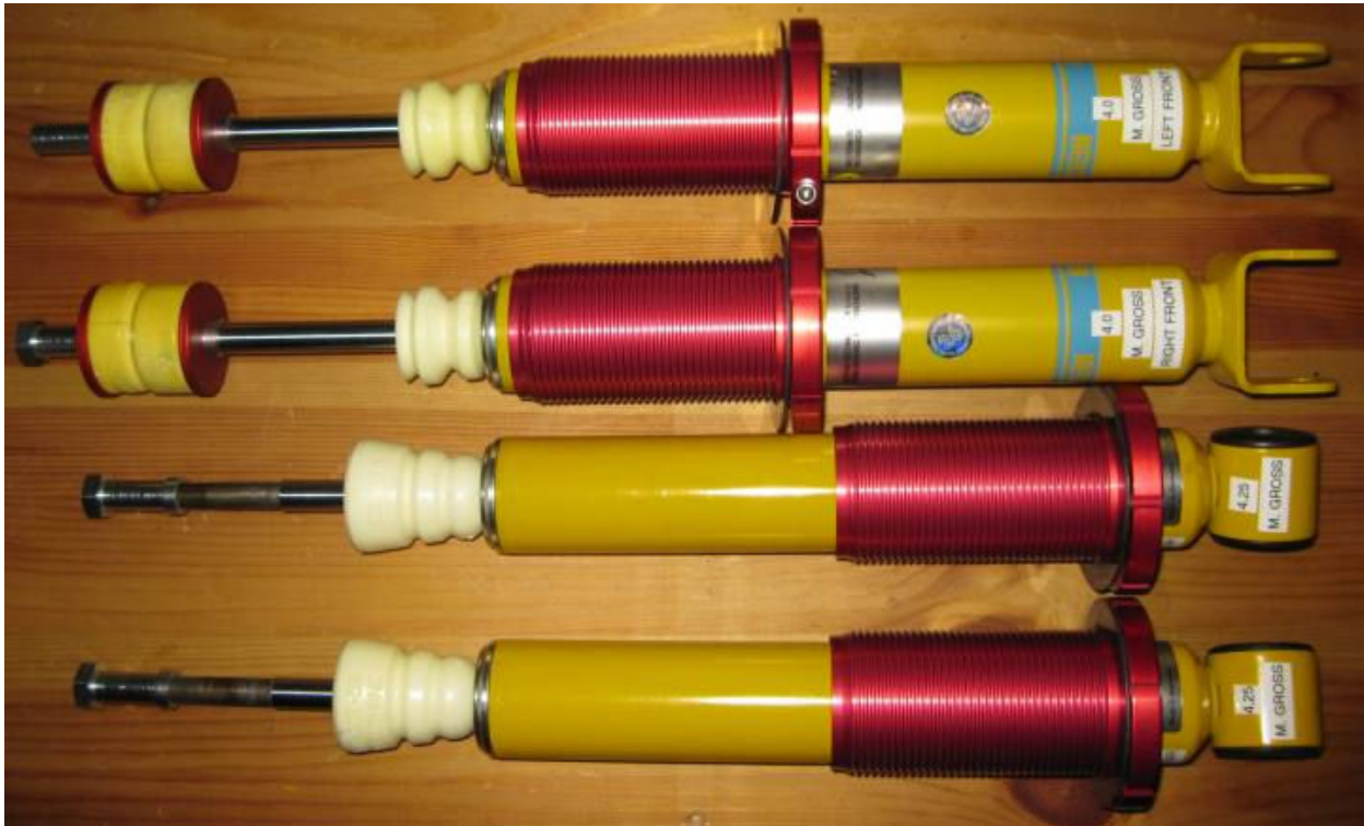
Figure 1a. Unassembled NC (2006+) MX5 Miata FCM Variant 2 coilovers. MCU bushing (in yellow) shown on upper portion of front shocks – not provided in all cases
