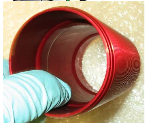
Figure 6. This end goes over the shock first
