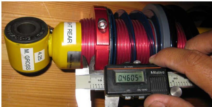
Figure 23. Rear lower spring perch nominal position
