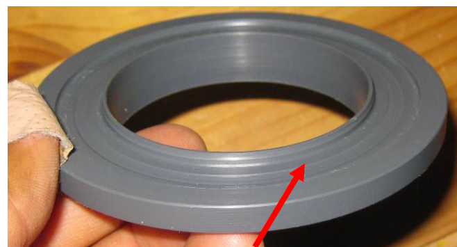
Figure 16. Bottom surface counterbored for 2.5" ID helper spring
