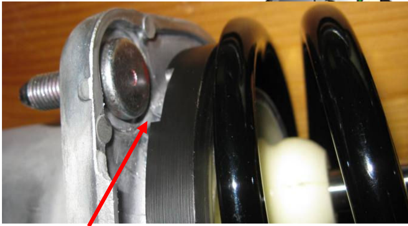
Figure 20. Notch in rear spring adapter to index against OE stud.
