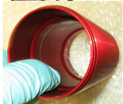
Figure 6. This end goes over the shock first
