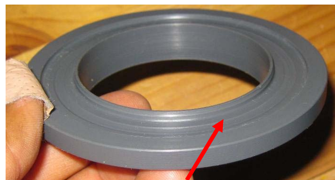
Figure 16. Bottom surface counterbored for 2.5" ID helper spring
