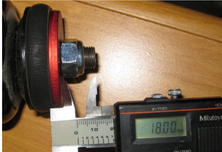
Figure 22. Measure this distance for proper bushing load (16-18mm)
