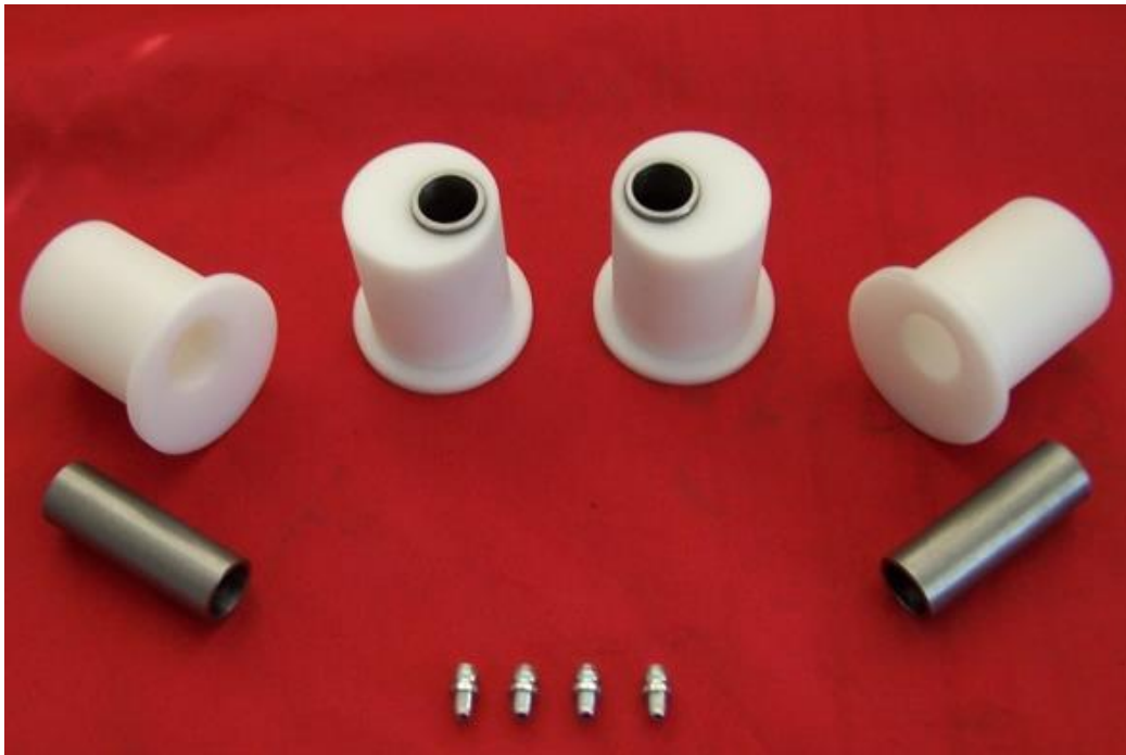
ISC Racing Delrin offset bushings, sold by Mazdaspeed Motorsports, installed on Senna’s front upper control arm bushing position
