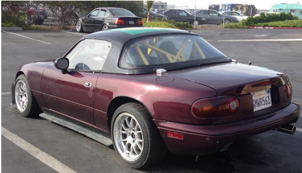
Lower section of rear bumper is cut to reduce 'parachute' effect from stock bumper
